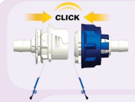
Align male and female couplings, push together until audible "Colder Click" confirmation. Slight rotation of lock ring may be required for proper alignment prior to connection.
